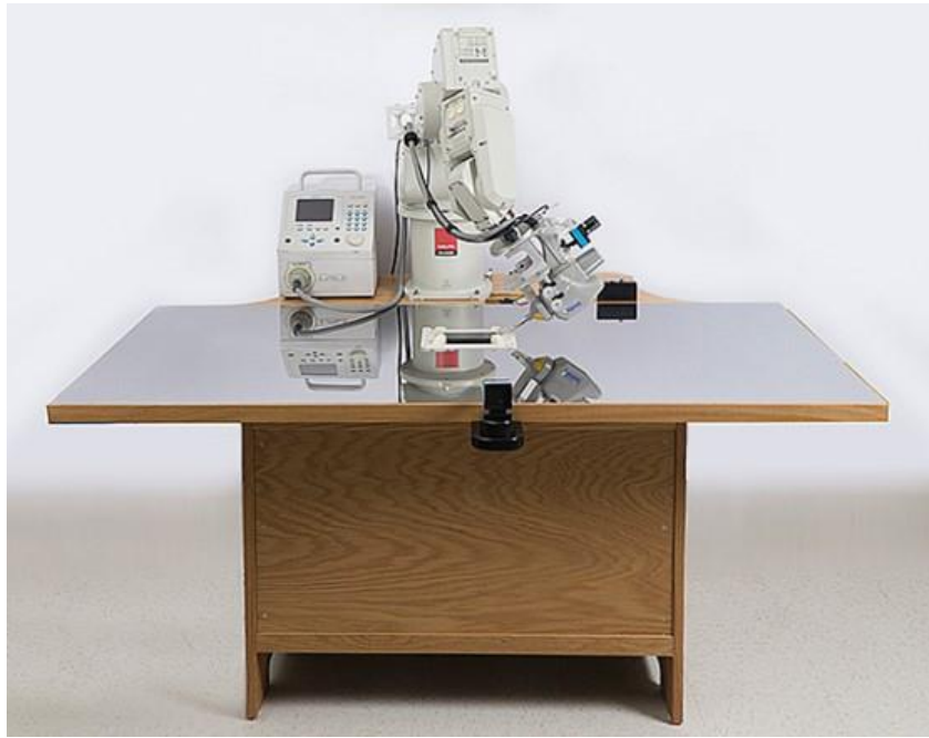
Figure 77: Robotic IEC 61000-4-2 test system (courtesy of API, www.amberpi.com )
