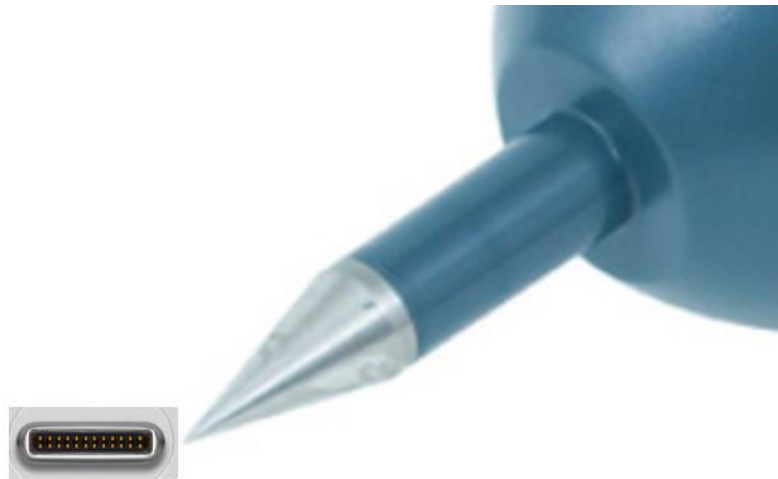
Figure 16: Comparison of a USB-C connector Size and the Tip of an IEC 61000-4-2 gun
