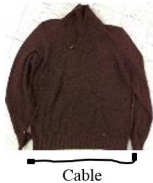
Figure 2: Rubbing of the sweater on the cable leads to a charge developed on the cable.
